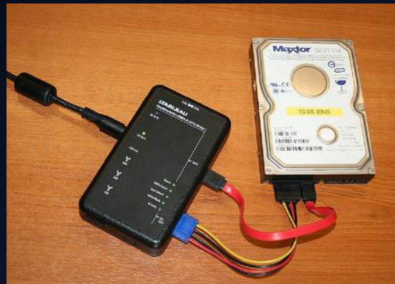
A portable Tableau write-blocker attached to a hard drive https://en.wikipedia.org/wiki/File:Portable_forensic_tableau.JPG
